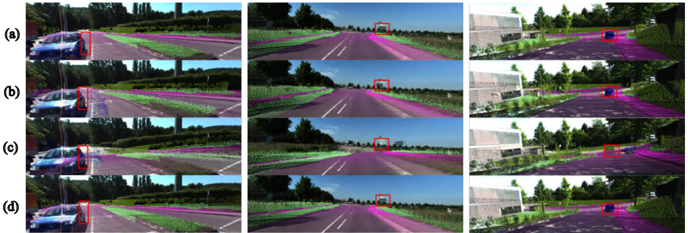
Fig. 5: (a) KIT360 calibration; (b) SOIC Results; (c) MI using surface intensities; (d) MI using semantic information.
